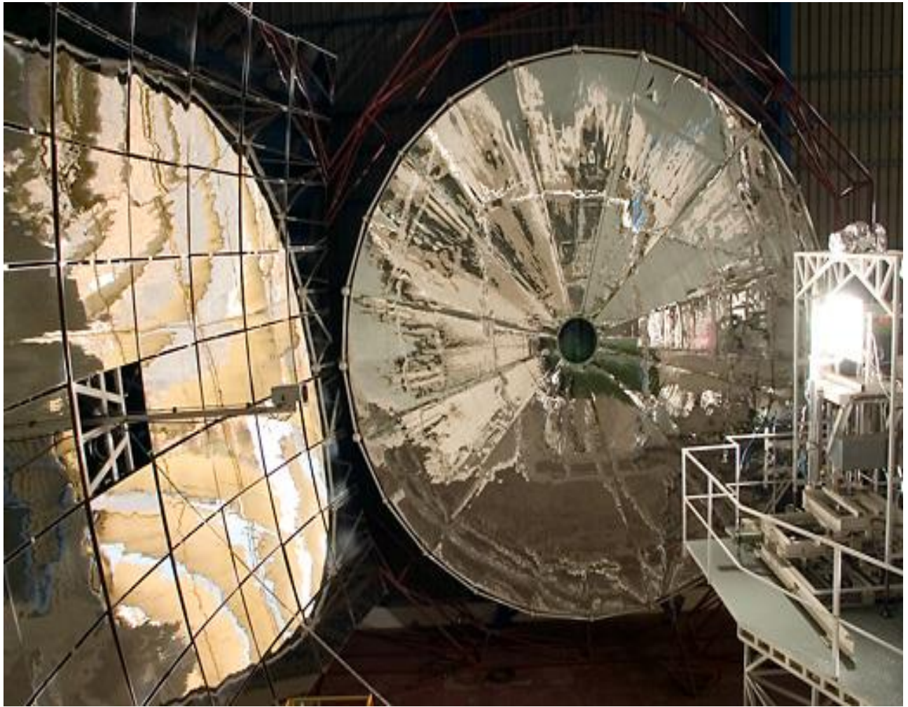
Figure 2.6 Solar furnace in Almeria, Spain; with the Concentrator (left) and receiver (right)[4].
